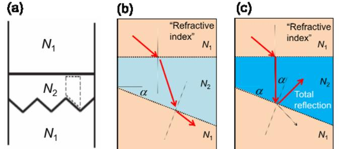
Fig. 1 (a) Schematic of zigzag-shaped npn junctions. (b, c) Schematic of mechanism of this device shown in the elementary unit of this device as depicted in dashed region in (a). Each represents (b) ON state at  $N_1 < N_2$  and (c) OFF state at  $N_1 \ll N_2$ .
