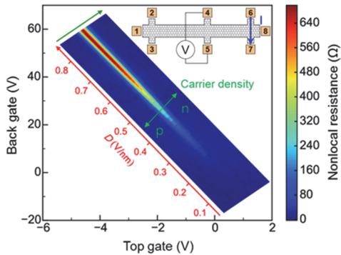
Fig. 3 Electric displacement field ( $D$ ) and carrier density dependence of the nonlocal resistance.  $D$  is tuned along the red arrow. Carrier density is tuned along the both ended green arrow. Inset: The configuration of nonlocal resistance measurement.
