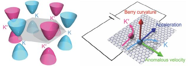
Fig. 1 (a) Band structure of gapped bilayer graphene. K and K' represent valley index. (b) Schematic image of the valley Hall effect.
