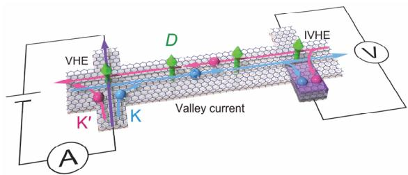
Fig. 2 Schematic image of the valley current mediated nonlocal transport and the setup of the nonlocal resistance measurement.
