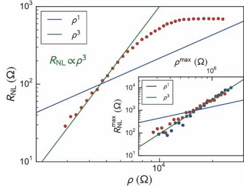
Fig. 4 Scaling relation between  $\rho$  and  $R_{NL}$  at the CNP by tuning  $D$ . Inset : Scaling relation obtained from other device. Red points and blue points are obtained from  $D > 0$  and  $D < 0$ , respectively.
