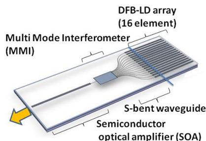
Fig. 1 A schematic of the tunable laser used in the measurement<sup>7</sup>
