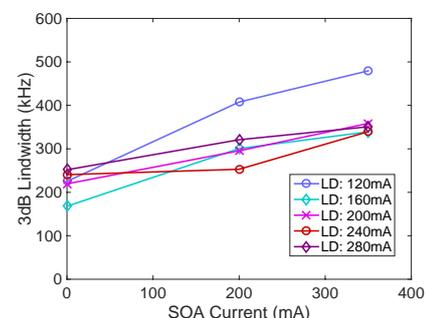
Fig. 2 Linewidth of the tunable laser as a function of the SOA current measured by the DSHI.
