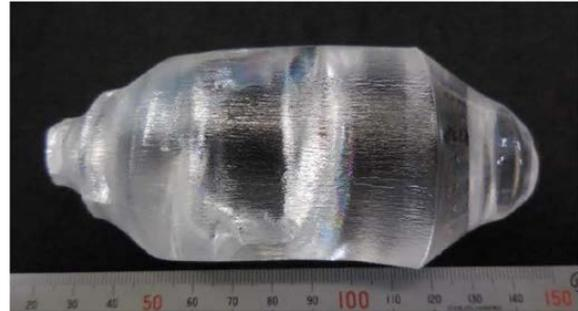
**Figure 1:**  $^{167}\text{Er}$  doped- $\text{Y}_2\text{SiO}_5$  ingot grown by Cz method
