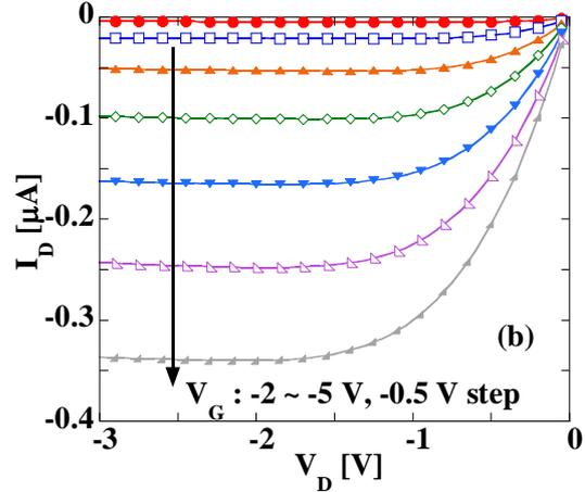
Figure 3 (a)  $I_D$ - $V_G$  and (b)  $I_D$ - $V_D$  characteristics of fabricated OFET with 2.2 nm-thick N-doped LaB<sub>6</sub> IL.
