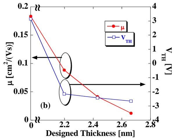
Figure 4 Thickness dependence of IL thickness on device parameters. (a) SS, and (b) mobility and  $V_{TH}$ .
