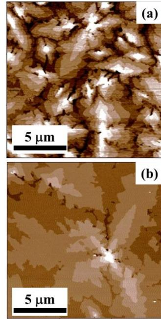
Figure 2 Surface morphology of pentacene film on (a) SiO<sub>2</sub> and (b) 2.7 nm-thick N-doped LaB<sub>6</sub> IL.
