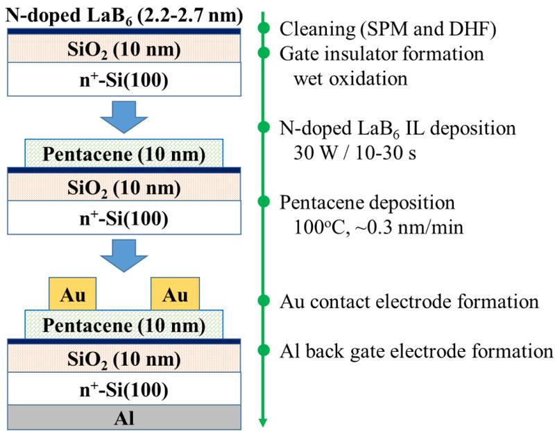
Figure 1 Experimental procedure of OFETs fabrication.
