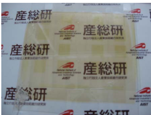
Figure 4a photograph of transparent sensor array sheet
