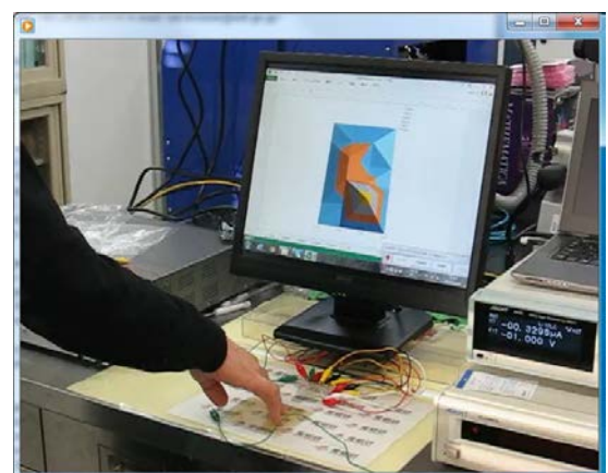
Figure 4b picture of visualization of the variation of currents for each sensor device
