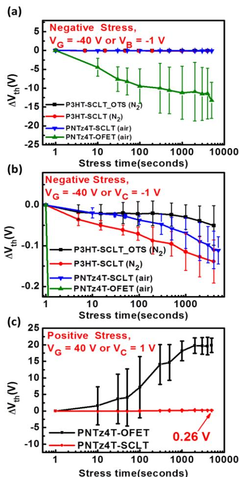
Fig. 3 Threshold voltage shift versus stress time under (a) negative base stress and (b) positive base stress. (c) The smaller scale figure of (a).
