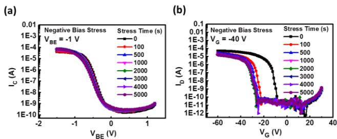
Fig. 2 Transfer characteristics with various bias stress time of (a) PNTz4T-SCLT and (b) PNTz4T-OFET.
