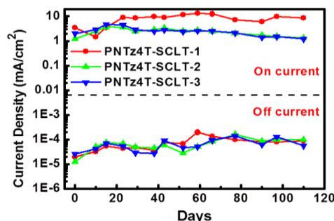
Fig. 4 Output current density against days of 3 PNTz4T-SCLTs.
