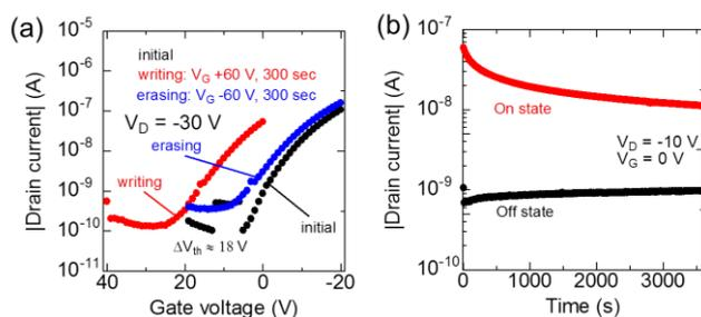
Fig. 5. (a) Writing and erasing, and (b) retention characteristics of top-gate P3HT OFET memory with PMMA:PCBM (97:3) composite film.
