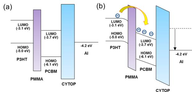
Fig. 4. Energy band diagrams of TG/BC P3HT FET memory with PMMA:PCBM composite film for (a) initial state and (b)  $V_G > 0$ .
