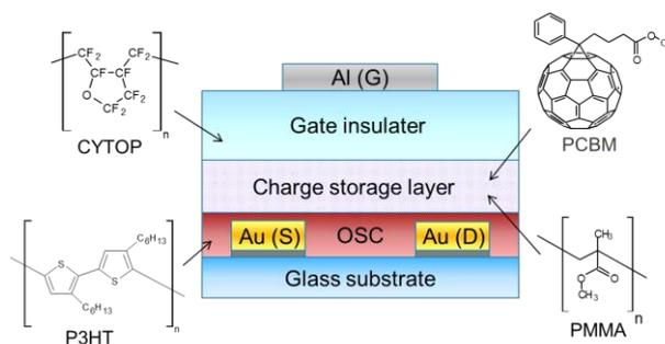
Fig. 1. Schematic structure of solution-processed TG/BC OFET memory device.
