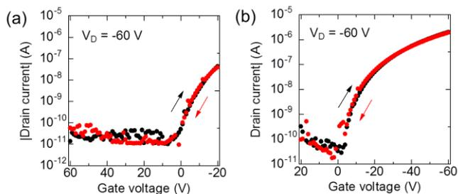
Fig. 2. Transfer characteristics of fabricated TG/BC P3HT FET memory with PMMA/CYTOP double layers measured at (a)  $V_G = 60 \sim -20$  V and (b)  $20 \sim -60$  V.
