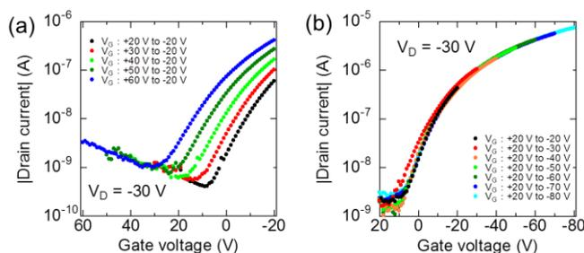
Fig. 3. Transfer characteristics of fabricated top-gate P3HT FET memory with PMMA:PCBM composite film measured for (a) positive and (b) negative  $V_G$  applications.
