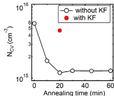
**Fig. 4** The  $N_{cv}$  as a function of annealing time for the CIGS solar cell fabricated without (open circles) and with KF-PDT process.
