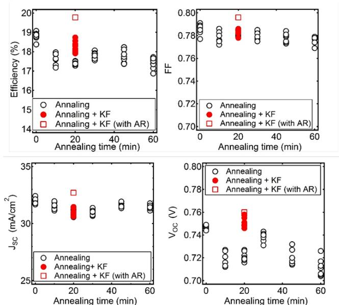
**Fig. 2** Photovoltaic properties for CIGS solar cells which underwent annealing (open circles) and KF-PDT, i.e. annealing with KF flux (closed circles). A solar cell had an anti-reflection (AR) coating (open squares).
