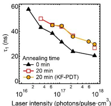
**Fig.3** Estimated minority carrier lifetimes for the CIGS thin films covered with CdS buffer layer as a function of laser intensity. The lifetimes were estimated by fitting TRPL decay curves by double exponential model. The shorter ( $\tau_1$ ) lifetime components were shown.
