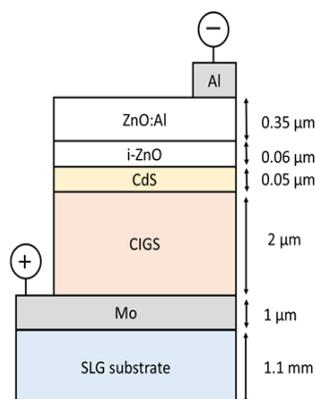
**Fig. 1** Schematic structure of CIGS solar cell fabricated in this work. The substrate was soda lime glass (SLG). The total area of a cell was 0.519 cm<sup>2</sup>.
