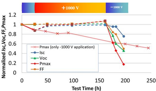
Fig. 3 Normalized  $I_{sc}$ ,  $V_{oc}$ , FF and  $P_{max}$  as a function of test time. Blue and red bars show -1000 V and +1000 V applications, respectively.
