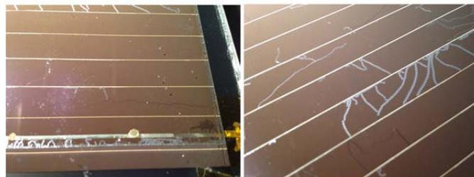
Fig. 2 Photographs of the examples of the delamination observed after PID test over 150 h.
