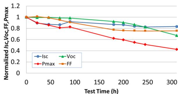
Fig. 1 Normalized  $I_{sc}$ ,  $V_{oc}$ , FF and  $P_{max}$  as a function of PID test time.
