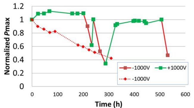
Fig. 5 Normalized  $P_{max}$  as a function of time for alternate test of +1000 V and -1000 V applications. Normalized  $P_{max}$  as a function of time for test of only -1000 V application is shown for comparison.
