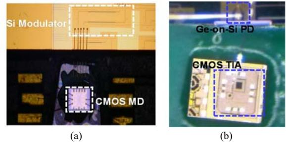
Fig. 5. Wire bond integration of (a) silicon optical modulator with 90-nm CMOS DA. (b) Ge-on-Si PD with 90-nm CMOS TIA.
