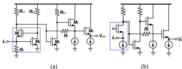
Fig. 2. (a) TIA with the regulated cascode (RGC) input stage (b) TIA with the common-gate (CG) input stage.
