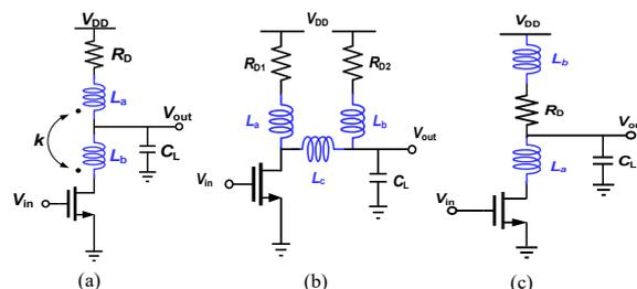
Fig. 3. Different inductive peaking topologies (a) T-coil peaking (b)  $\pi$ -type inductor peaking (c) reversed triple resonance network (RTRN).
