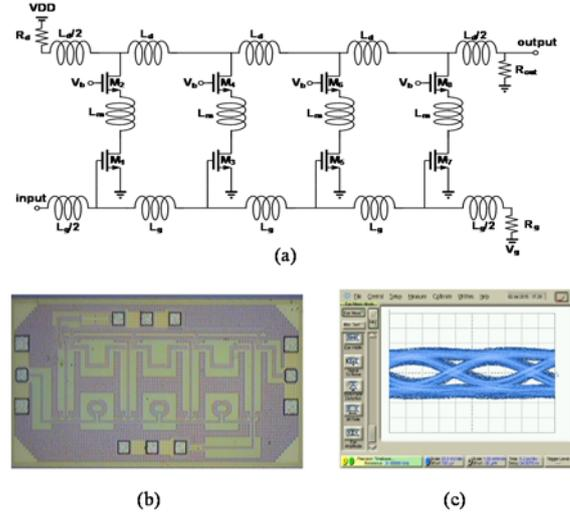
Fig. 4. (a) Proposed circuit topology of distributed amplifier (DA) in 90-nm CMOS (b) chip micrograph (c) measured eye diagram at 40 Gb/s.
