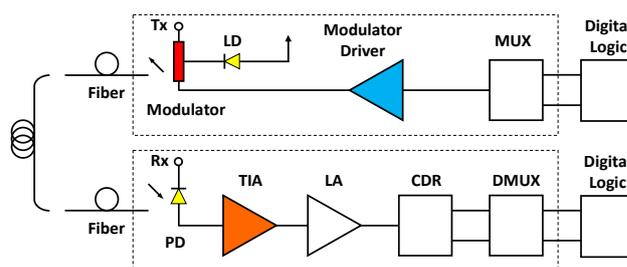
Fig. 1. Typical optical communication system, where the TIA/PD and modulator driver/modulator are very critical for achieving high-speed data transmission.
