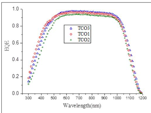
Fig. 3 External quantum efficiencies of SHJ solar cells with various TCO films
