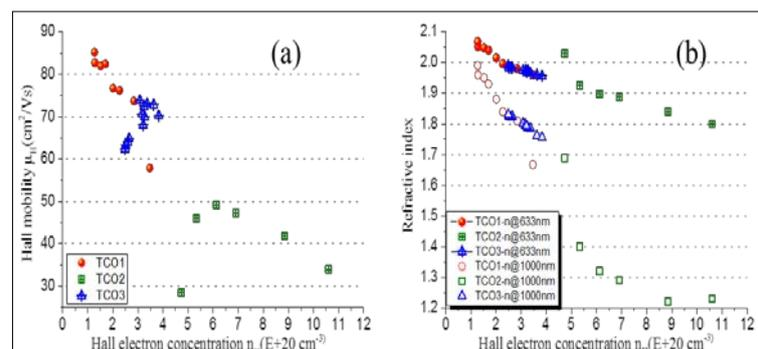
Fig.1 TCO material parameters (a)  $\mu_H$  vs. electron concentration; (b)  $n$  vs. electron concentration.
