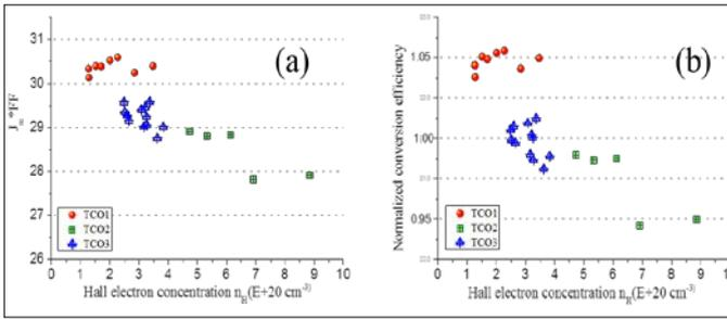
Fig. 2 Dependence of SHJ solar cell parameters on hall electron concentration, (a)  $J_{sc} * FF$  vs. electron concentration; (b) normalized efficiency vs. electron concentration.
