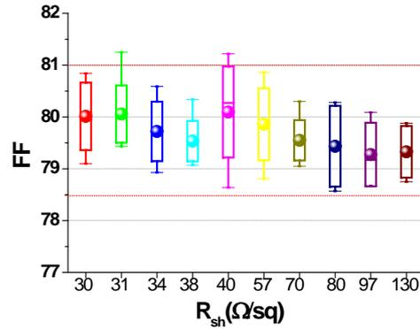
Fig.4 Dependence of *FF* on sheet resistance ( $R_{sh}$ ) of TCO films
