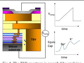
Fig 4. The TVS spectrum is recorded by applying a ramp voltage and recording the current, typically expressed as an equivalent capacitance; lighter ions such as  $Na^+$  typically show up earlier and have sharper peaks than heavier ions such as  $K^+$  or  $Cu^{++}$
