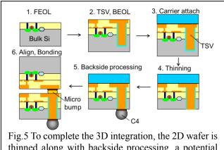
thinned along with backside processing, a potential source for the introduction of ions. This can pose additional sources of perturbation to devices.
