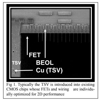
alone 2D chips (Fig1). However, the high aspect ratios involved in the TSV along with challenges introduced due to process can perturb the functionality of the CMOS layer. In this paper, we discuss such a perturbation, one that is related to electrostatic charges resulting from TSV process.
