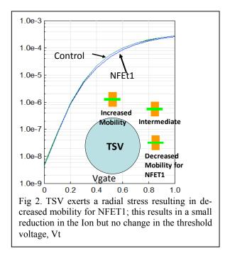
in the reduction of the ion of NFET1 (Fig 2) while no change is observed in the threshold voltage (Vt). However, if there are positive charges present in proximity, either through mobile ion contamination [2] or copper extrusions [3], the threshold voltage is changed (Fig 3).
