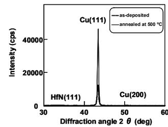
Fig. 1 XRD patterns of Cu(100 nm)/HfN<sub>x</sub>(5 nm)/SiO<sub>2</sub>/Si system before and after annealing at 500 °C 1h..
