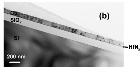
Fig. 3 Cross-sectional TEM images of Cu(100 nm)/HfN<sub>x</sub>(5 nm)/SiO<sub>2</sub>/Si system before annealing: (a) local view, and (b) entire view.
