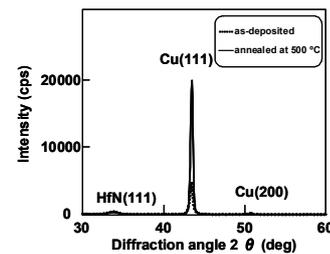
Fig. 2 XRD patterns of Cu(100 nm)/HfN<sub>x</sub>(10 nm)/SiO<sub>2</sub>/Si system before and after annealing at 500 °C 1h..
