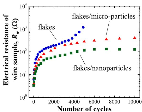
Fig. 2 Variation in electrical resistance of stretchable printed wire samples using single- and bimodal conductive pastes at the loading state during a uniaxial cyclic tensile test at 10 % strain.
