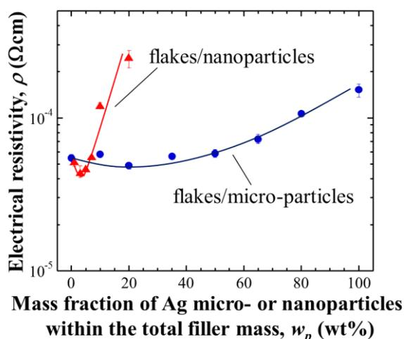
Fig. 1 Electrical resistivity of printed wire samples using bimodal conductive pastes with no tensile strain, as a function of mass fraction of Ag micro- or nanoparticles within the total filler loading.
