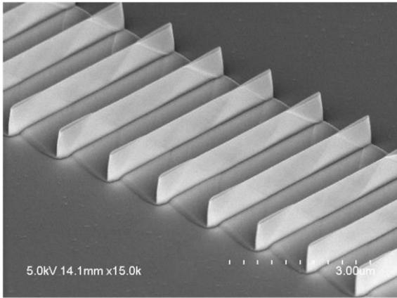
Fig. 3 SEM images of an array of InP fins formed by i-MacEtch.
