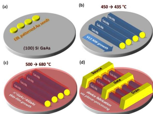
**Fig. 1** Process flow for the growth and fabrication of planar GaAs NW HEMT with AlGaAs:Si carrier supplying layer and n<sup>+</sup>GaAs cap.
