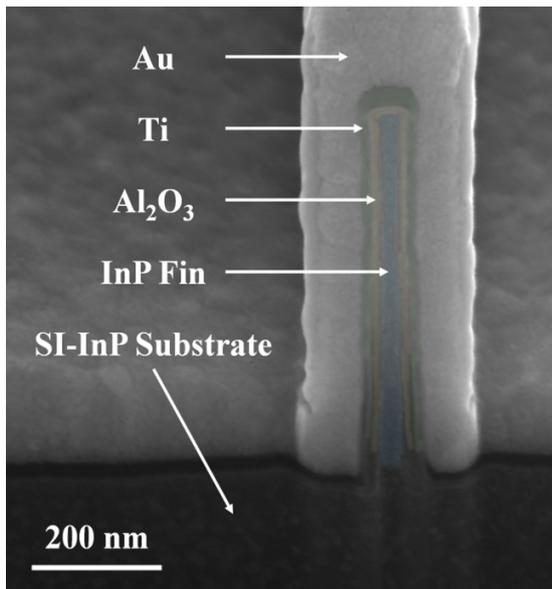
Fig. 4 SEM of a fully fabricated InP fin with fin width as narrow as 14 nm and height of 700 nm. Adapted from ref. [5].
