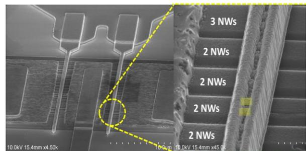
**Fig. 2** SEM image of a fully fabricated double-channel T-gated GaAs/AlGaAs NW HEMT, with the NW-channel region zoomed in where the T-gate can be seen sitting atop groups of parallel NWs.
