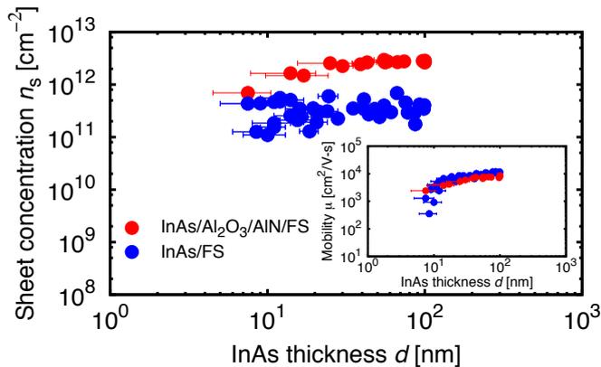
Fig. 2: Electron sheet concentrations  $n_s$  and mobilities  $\mu$  as functions of InAs thickness  $d$ .
