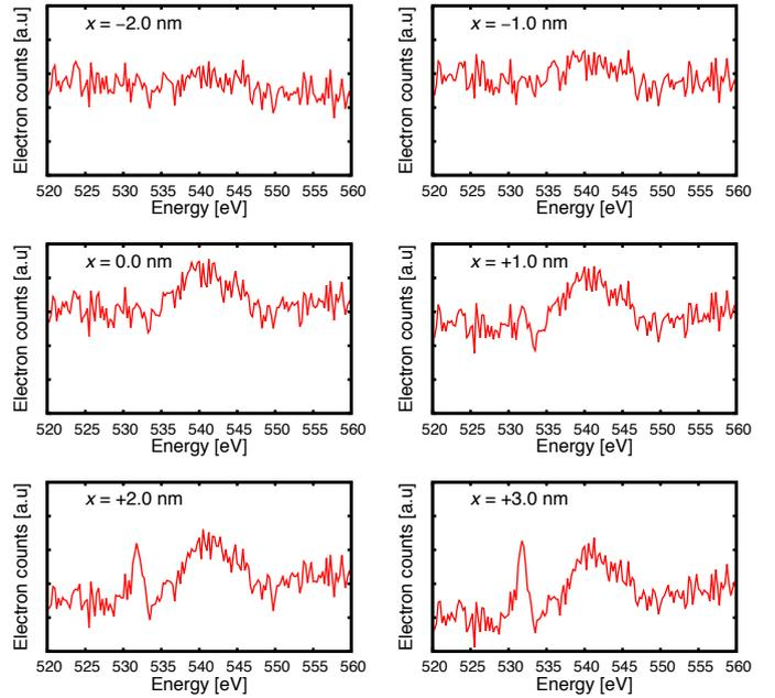
Fig. 4: EELS spectra for the position  $x = -2$ +3 nm.
