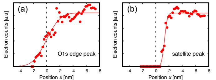
Fig. 5: (a) O1s edge peak and (b) satellite peak heights as functions of the position  $x$ .
