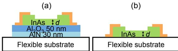
Fig. 1: Schematics of Hall-bar devices obtained from (a) InAs/Al<sub>2</sub>O<sub>3</sub>/AlN/FS and (b) InAs/FS.
