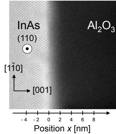
Fig. 3: A HAADF STEM image of the InAs/Al<sub>2</sub>O<sub>3</sub> interface.
