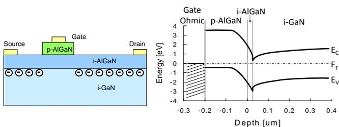
Fig. 4 A schematic cross section and operating principle of GIT.
