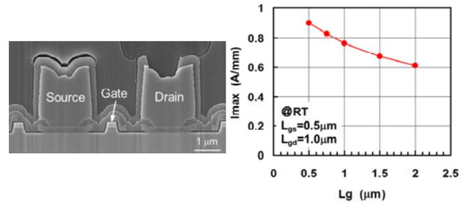
Fig. 5 SEM cross section of GIT with gate length (Lg) of 0.5 μm and Ids dependence on Lg.
