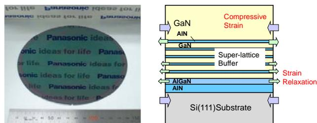
Fig. 1 Photograph of epitaxially grown AlGaIn/GaN hetero structure on Si substrate and schematic structure of buffer layer.
