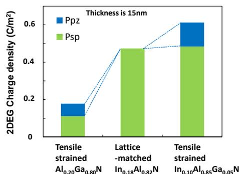
Fig. 2 Comparison of induced charge density of 2DEG for AlGaIn/GaN, InAlN/GaN and InAlGaIn/GaN.
