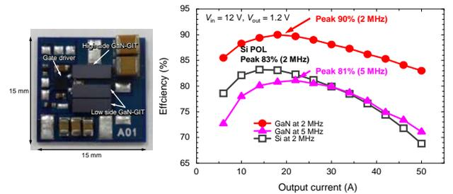
Fig.6 Photograph of DC/DC converter module and the frequency dependence of measured efficiency as a function of operation current.
