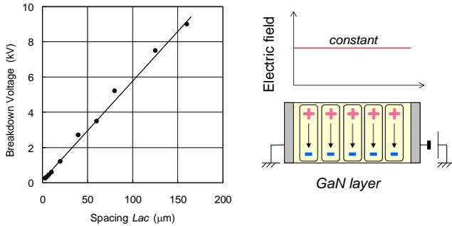
Fig. 3 The model of a single layer of GaN in which the polarization charges on front and back side are canceled.
