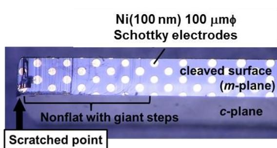
Fig. 2 Optical microscope image of Ni metal dots on a cleaved n-GaN surface.
