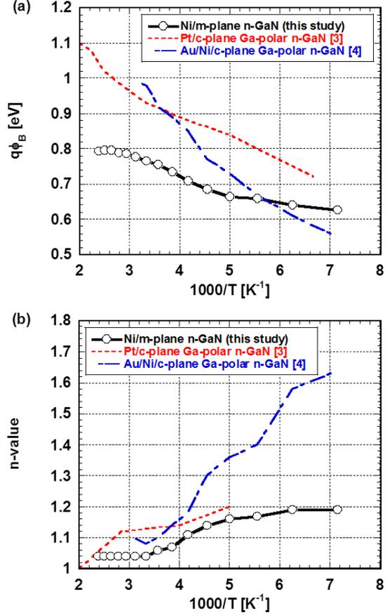
Fig. 4 Temperature dependences of (a)  $q\phi_B$  and (b)  $n$ -value obtained from forward  $I$ - $V$ - $T$  results of the Ni/ $m$ -polar n-GaN contacts, comparing with reported values of  $c$ -plane Ga-polar n-GaN contacts.
