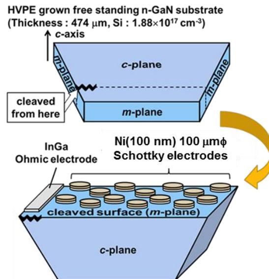
Fig. 1 Device structure.
