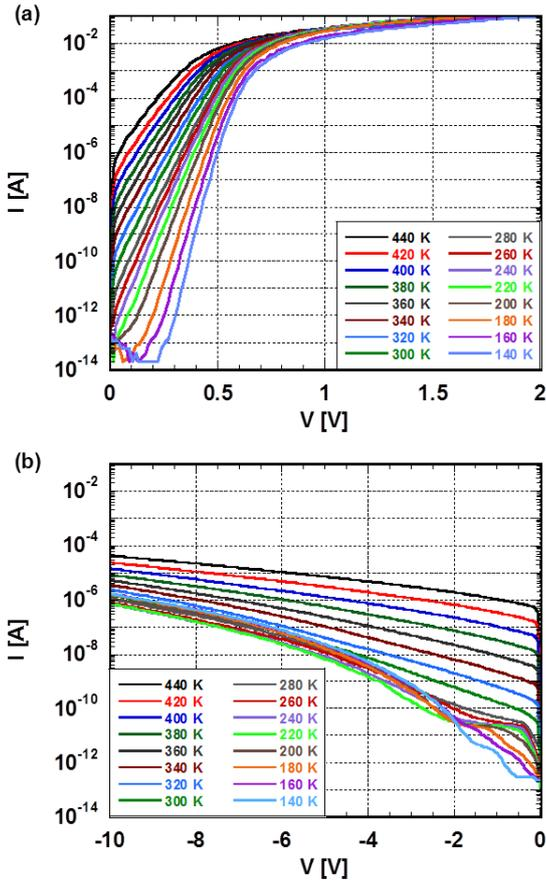
Fig. 3 (a) Forward and (b) reverse  $I$ - $V$ - $T$  characteristics of the Ni/ $m$ -plane n-GaN Schottky contacts.
