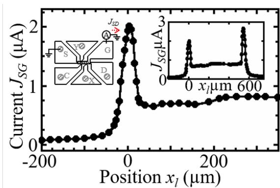
Fig. 2 Photocurrent  $J_{SG}$  as a function of laser spot position  $x_l$ .
