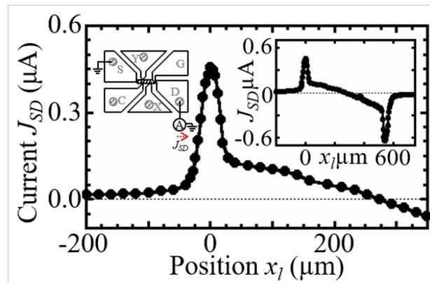
Fig. 3 Photocurrent  $J_{SD}$  as a function of laser spot position  $x_l$ .
