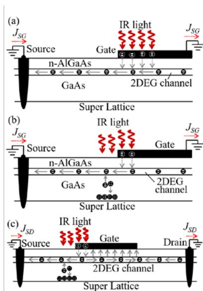
Fig. 1 Schematic drawings of the FET cross section views.
