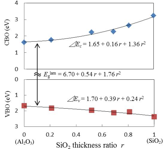
Fig. 4 The band offsets between  $\text{Al}_2\text{O}_3/\text{SiO}_2$  nano-laminate and GaN as a function of  $\text{SiO}_2$  thickness ratio  $r$ .
