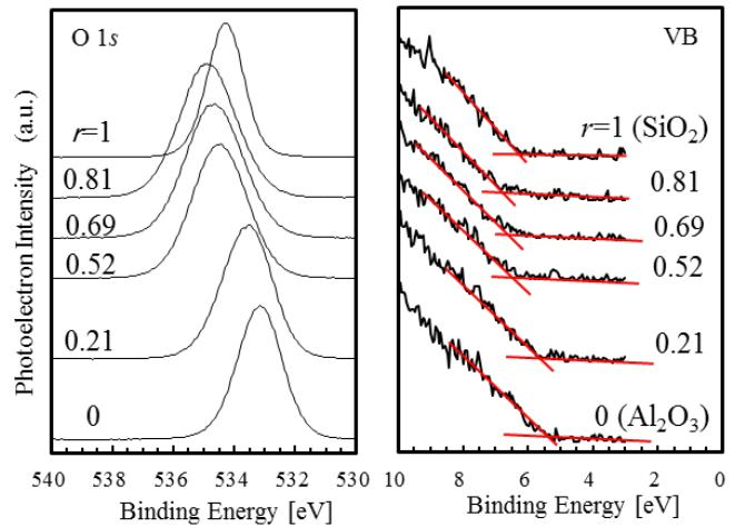
Fig. 3 Oxygen 1s core levels and valence band spectra of  $\text{Al}_2\text{O}_3/\text{SiO}_2$  nano-laminates with various  $\text{SiO}_2$  thickness ratios  $r$ .
