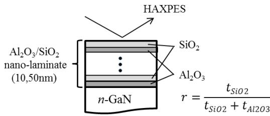
Fig. 1 Sample structure of an  $\text{Al}_2\text{O}_3/\text{SiO}_2$  nano-laminate on n-GaN.  $\text{SiO}_2$  thickness ratio in the nano-laminate was denoted as  $r$ .
