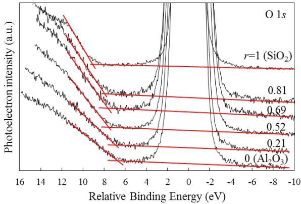
Fig. 2 Oxygen 1s plasmon loss spectra of  $\text{Al}_2\text{O}_3/\text{SiO}_2$  nano-laminates with various  $\text{SiO}_2$  thickness ratios  $r$ .
