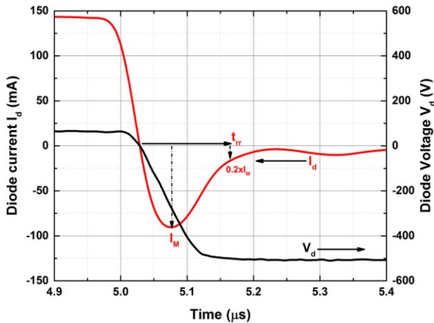
**Figure 2: Reverse-recovery waveforms of the diamond pin diode**
