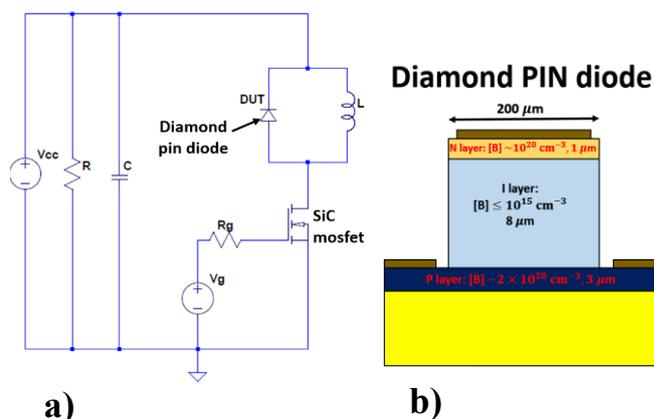
Figure 1: a) clamped inductive switching circuit, b) diamond pin diode structure
