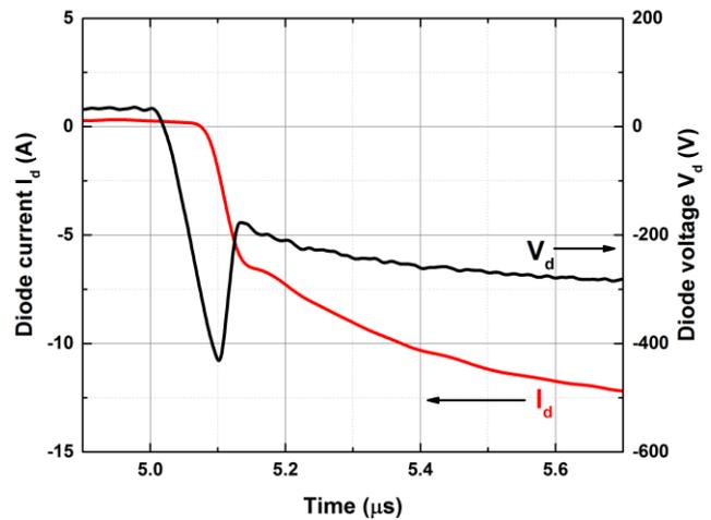
**Figure 3: dynamic breakdown of the diamond pin diode**
