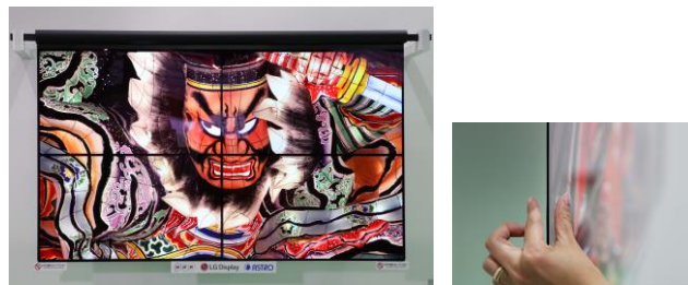
Fig. 5 130-inch Sheet-type OLED display (Cooperation with LG Display Co., Ltd. and Astrodesign Inc.,)
