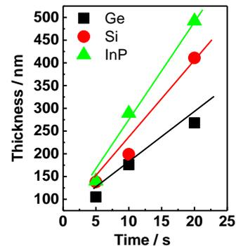
Fig. 10 Selective Ni growth on Si and InP substrates with electrodeposition.
