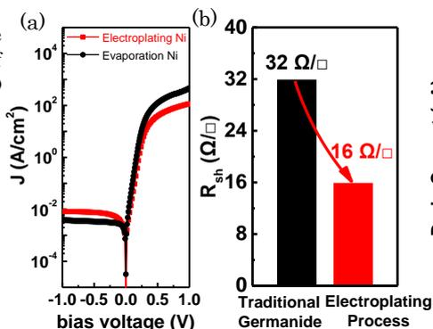
Fig.6 (a) I-V characteristics of electroplated Ni and thermally evaporated Ni with n- Ge and (b) sheet resistance( $R_{sh}$ ) comparison between electroplated Ni device and the traditional germanide device.
