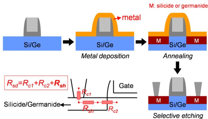
Fig. 1 Schematic diagram of silicide/germanide process.
