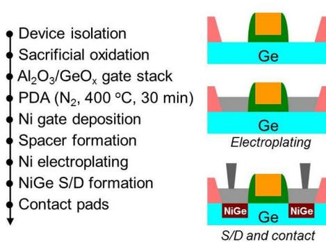
Fig.2 Process flow diagram of Ge pMOSFETs with electrodeposited Ni as contact metal in S/D region.
