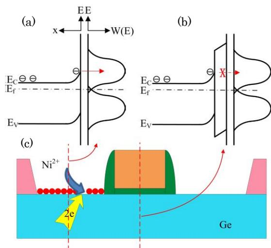
Fig. 3 The energy band diagram for the (a)S/D and (b)gate region in contact with a solution.(c)Schematic diagram of electrodeposition process for selective Ni deposition at S/D region of Ge MOSFET.
