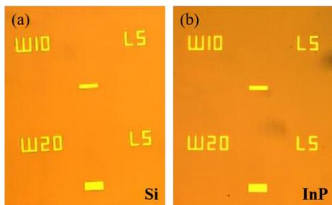
Fig.8 Microscope image of Ni selectively deposited on (a) Si and (b) InP substrates.
