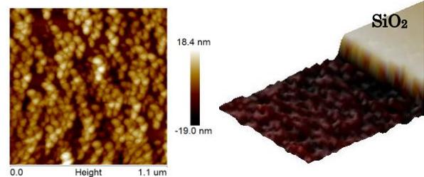
Fig. 5 AFM of (a) electroplated Ni film surface and (b) the step between Ni film and SiO<sub>2</sub> field oxide.
