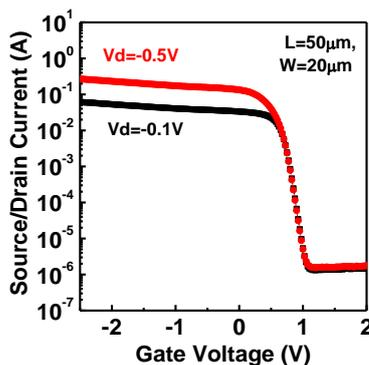
Fig.9 Device characteristics of metal source/drain Si pMOSFET with electrodeposited Ni.
