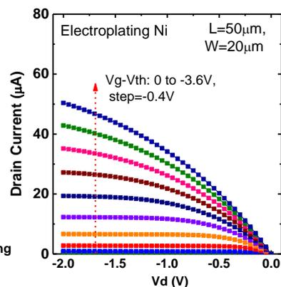
Fig.7 I-V characteristics of metal source/drain Ge pMOSFET with electrodeposited Ni.
