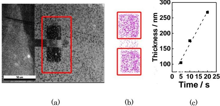
Fig. 4 (a) SEM image, (b) Mapping of Ni by EDS spectrum and (c) growth rate of selectively grown Ni at source/drain region of Ge pMOSFET.
