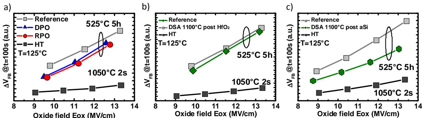
**Fig.4:**  $V_{FB}$  shift induced by negative gate bias. a) Slight improvement of reliability is obtained using plasma oxidation to stabilize the chemical oxide IL; b) almost no improvement is obtained with DSA milliseconds anneal on  $\text{HfO}_2$ ; c) more significant improvement can be obtained with DSA on LPCVD aSi.
