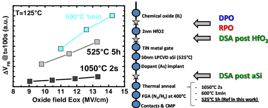
**Fig.1:** Flatband voltage shift induced by negative gate bias measured on MOS capacitors ( $50\mu\text{m} \times 50\mu\text{m}$ ). Low thermal budget leads to a strong degradation of reliability.
