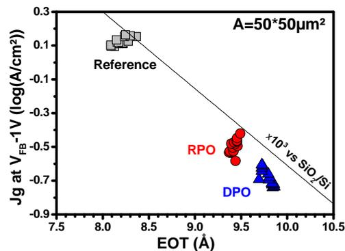
**Fig. 3:** Gate leakage current versus EOT. Plasma oxidation induced circa  $1\text{Å}$  thickening of the chemical oxide.
