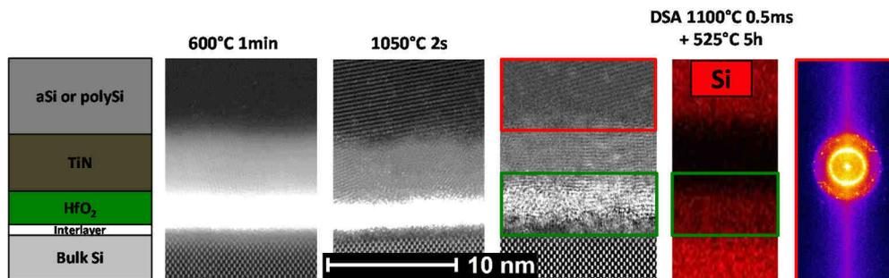
**Fig.6:** High resolution HAADF (Z-contrast imaging) cross-sectional scanning TEM observations of gate stacks annealed with different thermal budgets. Polycrystalline grains can be observed after a  $1050^\circ\text{C}$  2s or DSA  $1100^\circ\text{C}$  0.5ms anneal. In the latter case, amorphous phases are still present, as indicated by the rings observed in the numerical diffraction pattern of the capping silicon layer area. Besides, EDX measurements show formation of a Hf silicate.
