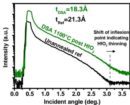
**Fig.5:** X-Ray Reflectometry measurements showing the densification effect of DSA annealing on  $\text{HfO}_2$  and confirmed by the thickness measured by ellipsometry.
