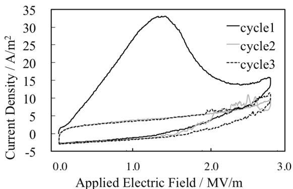
Fig. 4. J-E curves applied only positive voltage to P(VDF-TrFE)/PICPM-SCN gels for 3 cycles.
