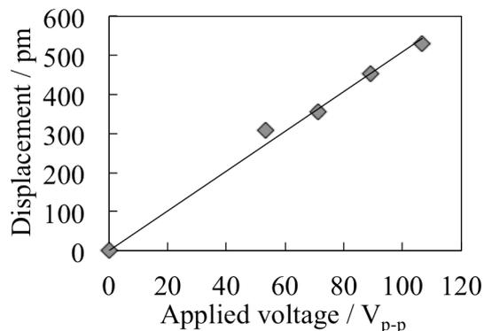
Fig. 5. Piezoelectric displacements of the P(VDF-TrFE)/PICPM-SCN gel at various applying voltages.
