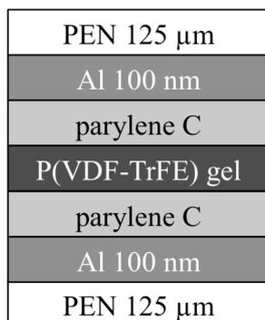
Fig.1. Device structure of P(VDF-TrFE)/PICPM-SCN gel.
