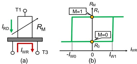
Figure 1. 3T-MTJ device: (a) structure, (b) R-I characteristic.
