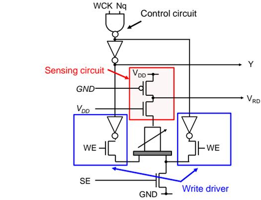
Figure 4. Schematic of the 3T-MTJ-based storage cell.
