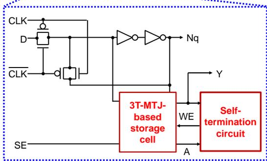
Figure 3. Schematic of the self-termination circuit.
