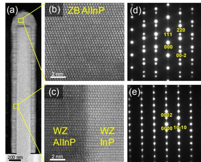
**Fig. 2** (a) Overall TEM image of the nanowire for  $X_{\text{TMAI}} = 0.18$ . High resolution TEM images (b) at the top of the nanowire and (c) at the interface of InP core and AlInP shell. The corresponding SAED patterns at the (d) top and (e) middle of the nanowire, showing a ZB structure and a WZ structure, respectively.
