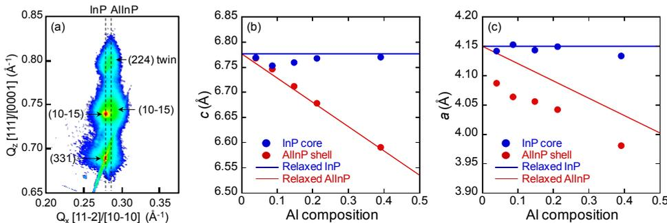
**Fig. 3** (a) XRD RSM of InP/AlInP core-multishell nanowires for  $X_{\text{TMAI}} = 0.18$ . (b) Axial and (c) radial lattice constants of the WZ InP core and AlInP shell calculated from the maximum peak position of (10-15) reflections. Blue and red solid lines represent the WZ lattice constants of relaxed InP and AlInP calculated from their ZB lattice constants when they are converted from ZB to ideal WZ.
