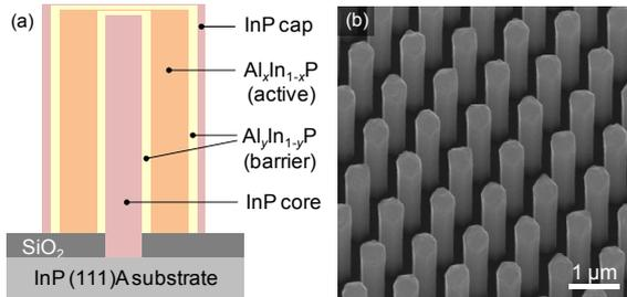
**Fig. 1** (a) Schematic view of grown layers of the core-multi shell nanowire. (b) 30°-tilted SEM image of the nanowires for  $X_{\text{TMAI}} = 0.18$ .
