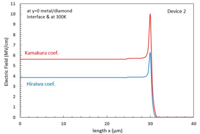
Fig. 4 Electric field peak at metal/diamond interface for the device 2 at 300K, at 230V for Hiraiwa model and at 490 for Kamakura's.
