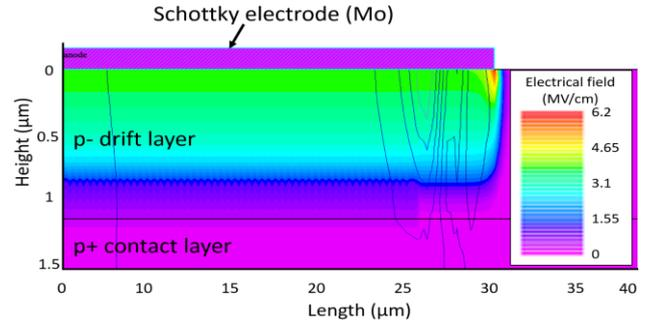
Fig. 3 Electric field map and current flowlines of simulated SBDs 2 just before the breakdown voltage (255 V) at 300°C
