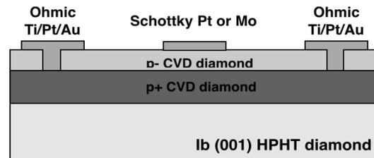
Fig. 1 Cross-sectional structure of fabricated diamond SBDs
