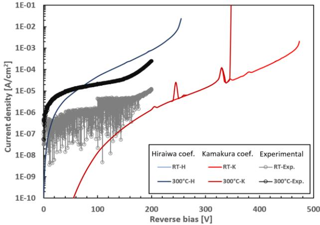
Fig. 2 b) Reverse conditions for experimental and simulated device 2 at different temperatures / Mo Schottky
