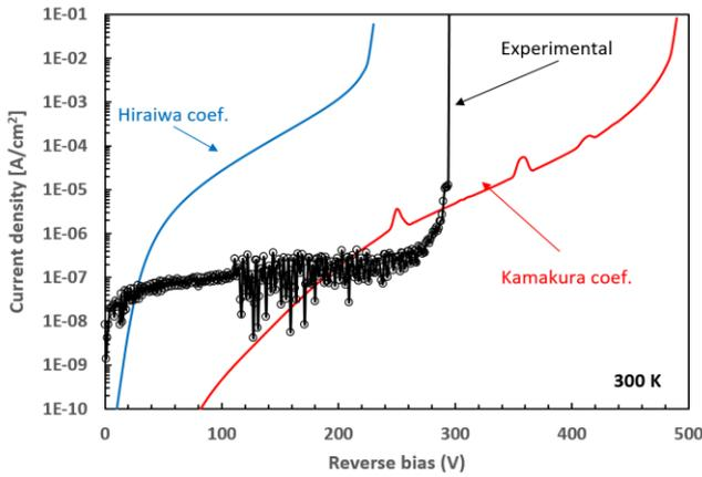
Fig. 2 a) Reverse conditions for experimental and simulated device 1 at Room Temperature (RT) / Pt Schottky
