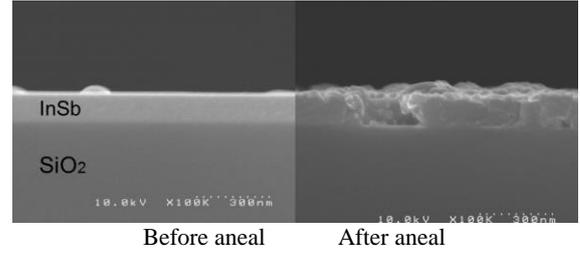
Fig.5 Cross-sectional SEM images of InSb film before and after annealing. (500°C, 30min)
