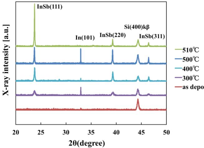
Fig.3 XRD  $2\theta$  scan of as deposited amorphous InSb, and poly-InSb formed by RTA annealing at different temperatures
