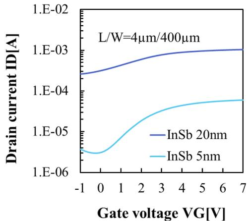
Fig.7  $I_d$ - $V_g$  characteristics of FLA poly-InSb nMOSFETs
