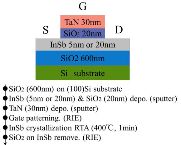
Fig.2 Schematic device structure and the process flow of poly-InSb nMOSFETs
