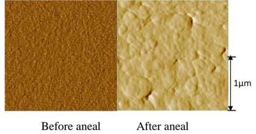
Fig.4 AFM images of InSb surface before and after thermal annealing. (500°C, 30min)
