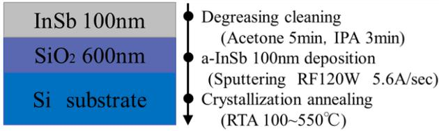
Fig.1 Schematic structure and process flow for fabricating poly-InSb thin films on Si.
