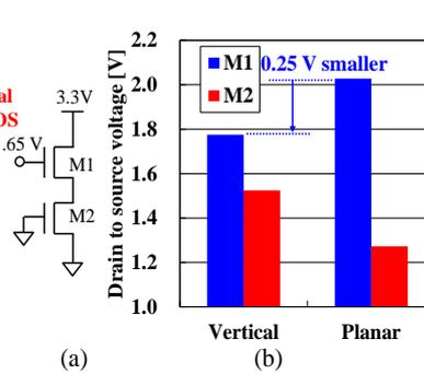
Fig. 8 (a) NMOS power switch in off-state and (b) comparison of voltage distribution between vertical and planar MOSFET.
