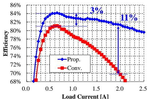
Fig. 10 Efficiency curve comparison of the proposed and conventional IVR.
