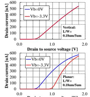
Fig. 6  $I_d V_g$  characteristics of vertical MOSFET comparison with planar MOSFET.
