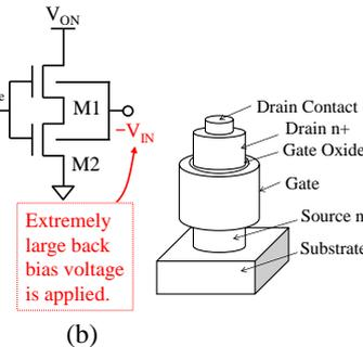
Fig. 5 Vertical MOSFET structure.
