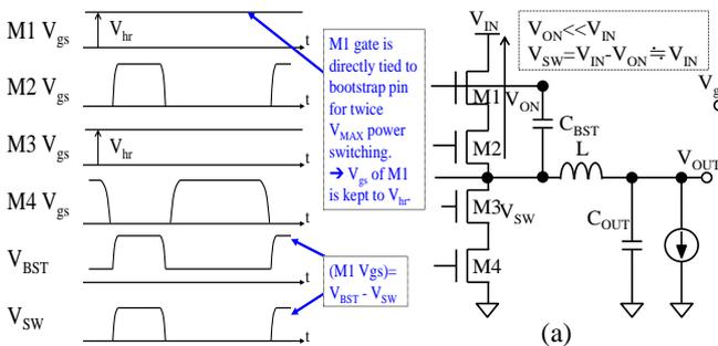
Fig. 3 Timing diagram of the proposed bootstrap driver for cascode bridge composed of HS NMOS power switch.
