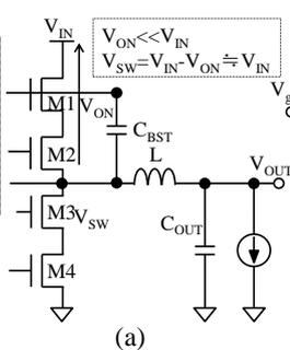
Fig. 4 (a) Voltage of terminals and (b) equivalent bias condition of HS NMOS power switch when on-state.
