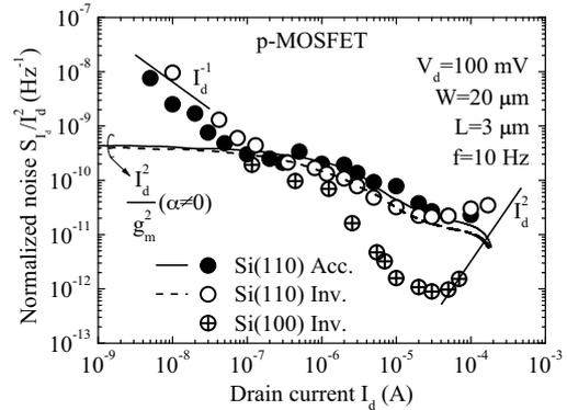
Fig. 5: Noise spectral density versus drain current of SOI accumulation- and inversion-mode p-MOSFETs fabricated on (100) and (110) silicon-oriented wafers.
