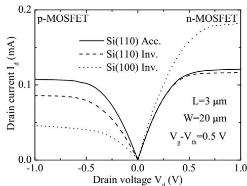
Fig. 2: Drain current versus drain voltage for SOI accumulation- and inversion-mode n- and p-MOSFETs when fabricated on (100) and (110) silicon-oriented wafers.
