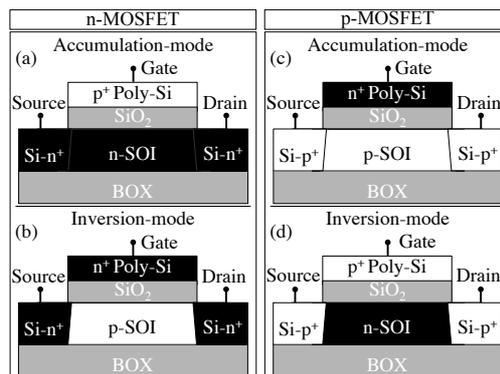
Fig. 1: Schematic of SOI accumulation- and inversion-mode n- and p-MOSFETs.
