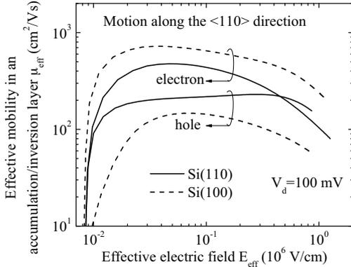
Fig. 3: Effective mobility versus effective electric field of hole and electron in an accumulation and inversion layer of MOSFETs fabricated on (100) and (110) silicon-oriented wafers. The channel is along the <110> direction.
