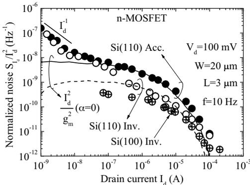
Fig. 4: Noise spectral density versus drain current of SOI accumulation- and inversion-mode n-MOSFETs when fabricated on (100) and (110) silicon-oriented wafers.
