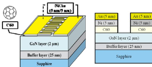
**Fig. 1** The schematic structure of GaN MOM UV PD with a C60 layer.
