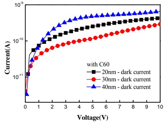
**Fig. 2** I-V characteristics of GaN MOM Sensors with C60 layers.
