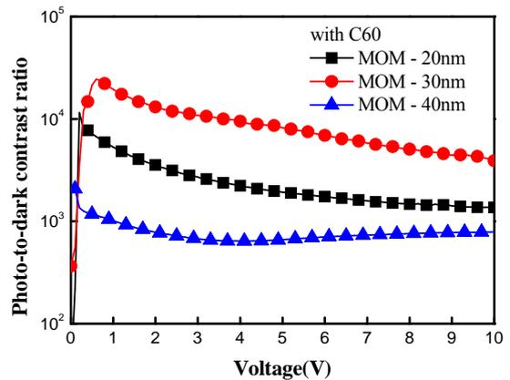
**Fig. 3** Photocurrent-to-dark current ratios of GaN MOM Sensors with C60 layers.
