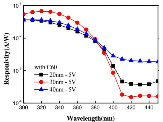
**Fig. 4** Spectral responses of GaN MOM Sensors with C60 layers.
