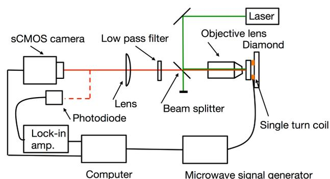
Fig. 1 Schematic diagram of a set-up for magnetic field imaging. Either an sCMOS camera or a photodiode is used.
