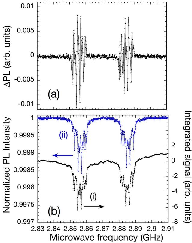
Fig. 2 (a) Frequency modulation signal obtained by a wide-field imaging using a 100x microscope objective as a function of the microwave frequency. (b) Integrated frequency modulation trace (i) and continuous-wave electron spin resonance trace (ii). Constant back-ground was corrected.
