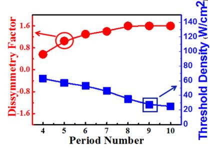
Fig. 4 Threshold density and the  $g_e$  factor against the periods of the left-handed metal/GaN double-spiral cavity.
