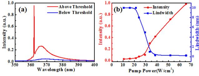
Fig. 2 (a) PL spectrum of the left-handed metal/GaN double-spiral cavity below (blue) and above (red) threshold (b) The Light-in and Light-out curve (L-L curve) and the linewidth variation from left-handed metal/GaN double-spiral cavity.
