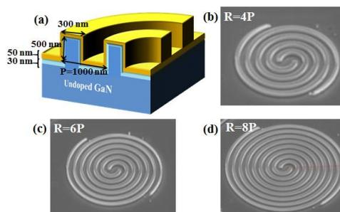
Fig. 1 (a) Schematic diagram of the metal/GaN double-spiral cavity. (b)(c)(d) The SEM image of the left-handed metal/GaN double-spiral cavity with different radius ( $R=4P$ ,  $6P$ ,  $8P$ ).
