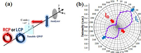
Fig. 3 (a) Schematic diagram of circularly polarized analyzer which can separate the LCP and RCP light by checking the direction of the linear polarization converted by the tunable quarter-wave plate. Degree of polarization of perpendicular and horizontal linear polarization light converted from the (b) L chirality laser (10 periods)
