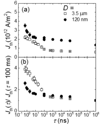
Fig. 2 (a)  $\tau$  dependence of  $J_{\text{th}}$  for dot devices with  $D = 3.5 \mu\text{m}$  and 120 nm. (b)  $J_{\text{th}}$  normalized by that at  $\tau = 100$  ms as a function of  $\tau$ .
