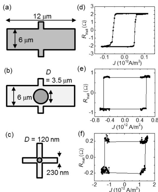
Fig. 1: (a)-(c) The schematics of three kinds of devices. (d)-(f) Corresponding SOT switching property, i.e., Hall resistance  $R_{\text{Hall}}$  versus current density  $J$ , where current pulses with  $\tau = 100$  ms are applied under 20-mT external field colinear with the current.
