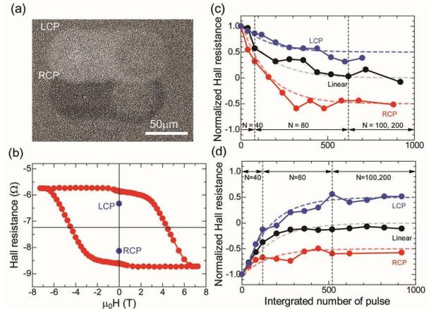
Fig. 1 Magnetization change observed from a FePt-C granular film by exposure to circular polarized light. (a) Magnetic image after exposure to RCP and LCP. (b) AHE curve for the FePt-C granular film. (c,d) Normalized Hall resistance after applying circular and linear polarized light.
