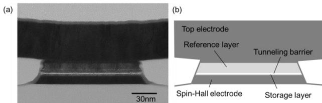
Fig. 2 A cross-sectional TEM image (a) and the schematic drawing (b) of the MTJ element and its electrodes.
