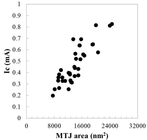
Fig. 4 MTJ area dependence of the critical switching current ( $I_c$ ) without VCMA. The measured current pulse width was 20 ns. The  $I_c$  was 200  $\mu\text{A}$  for a MTJ size of 7600 nm $^2$ .
