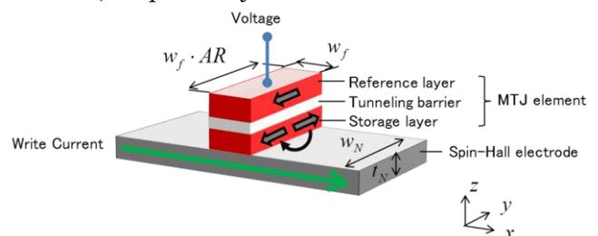
Fig. 1 A schematic drawing of VoCSM unit-cell, which has a MTJ element with a self-aligned spin-Hall electrode
