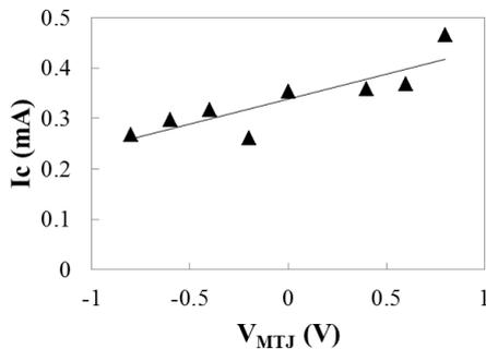
Fig. 3 The critical switching current ( $I_c$ ) as a function of  $V_{MTJ}$ .
