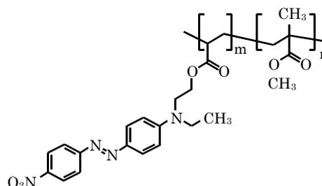
Fig. 2 Molecular structure of PMMA-co-DR1.
