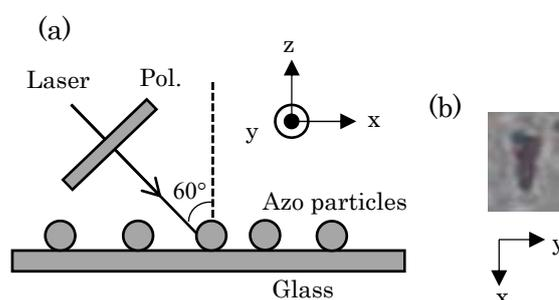
Fig. 5 Optical excitation of azo particles using oblique incidence of light illumination. The optical setup (a), and shape changes of azo particles with p-polarization (b).
