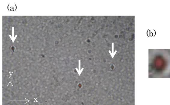
Fig. 4 Shape changes of azo particles after irradiation with the laser light at normal incidence. The particles were excited by the light with polarization in the y-direction (a), and re-excited using polarization in the x-direction (b).
