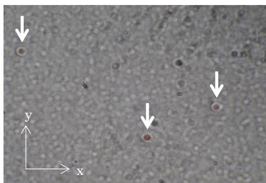
Fig. 3 Transmission optical microscopy image of azo particles generated by the colloidal method.
