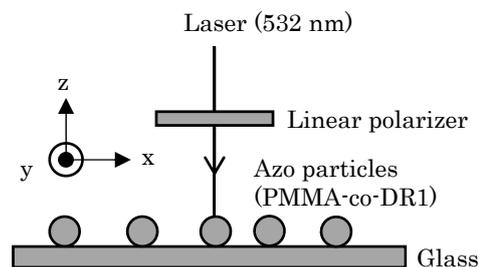
Fig. 1 Experimental setup.
