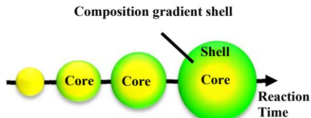
Fig. 1 Composition gradient shell growth using the reactivity difference between precursors
