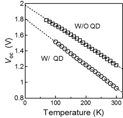
Fig.3  $V_{oc}$  in the InGaP-based InP QD (circles) and InGaP (squares) solar cells. Broken lines indicate the fitting results using Eq. (2).
