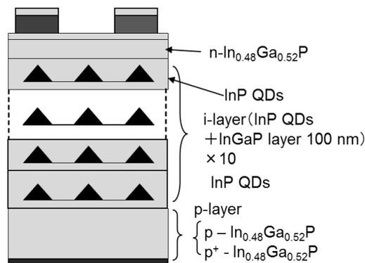
Fig.1 Schematic structure of the InGaP-based InP QD solar cells.
