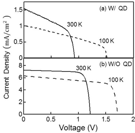
Fig.2 Current-voltage curves of the InGaP-based InP QD solar cells and (b) reference InGaP solar cells measured at 100 and 300 K.
