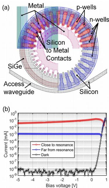
Fig. 4 | Resonance-enhanced photodiode. (a) The layout consists of a ring-resonator including a SiGe ring and T-shaped implants. (b) Illuminated and dark-current vs. bias voltage.
