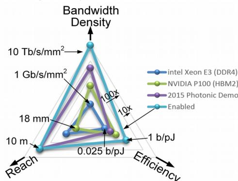
Fig. 2 | Radar chart of the I/O performance of state-of-the-art electronic and photonic links (legend). The scale is logarithmic and every line corresponds to a factor of ten.
