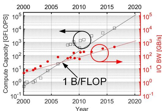
Fig. 1 | Evolution of single-precision floating-point compute capacity (black squares) and of the I/O bandwidth (red dots) of NVIDIA GPUs.
