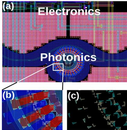
Fig. 3 | Design-Rule (DR) cleaning of a layout. (a) Electronic and photonic circuits are designed side-by-side with the same CAD tool. (b) Details of the microring resonator implant masks. (c) Same region as (b) showing the shapes which have been added/removed automatically by the DR-cleaning algorithm.
