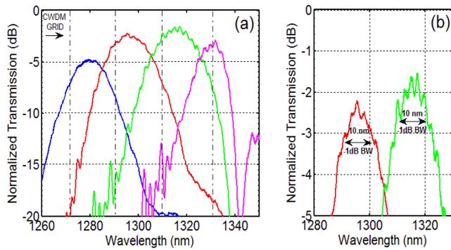
Fig. 2 (a) O-band 4 x 20 nm CWDM EG transmission spectrum (b) exhibiting a -1dB bandwidth of nearly 10 nm. Vertical dotted lines represent the nominal ITU grid.
