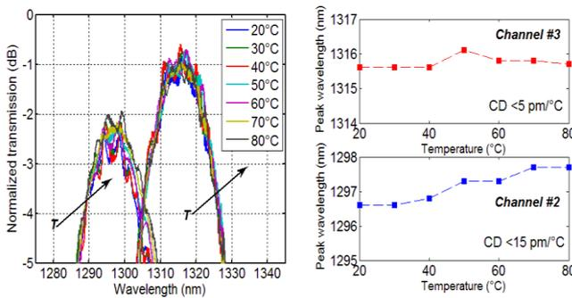
Fig. 3 (left) Temperature-dependent EG transmission spectra. (right) Channels #2 and #3 center wavelengths obtained from parabolic fitting. A close-to-zero thermal chromatic dispersion (CD) averaging 10 pm/°C is observed between 20 °C and 80 °C.
