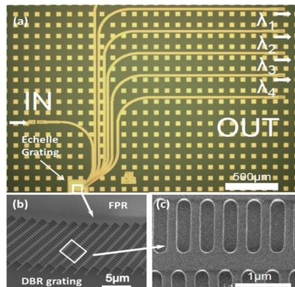
Fig. 1 (a) Optical microscope image of the CWDM4 EG demultiplexers on SiNOI using (b, c) 1<sup>st</sup>-order DBR-assisted facets for increased reflectance along the grating curve.
