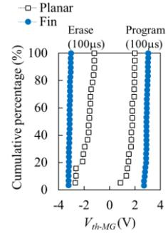
Fig. 7.  $V_{th-MG}$  distribution at P/E states.
