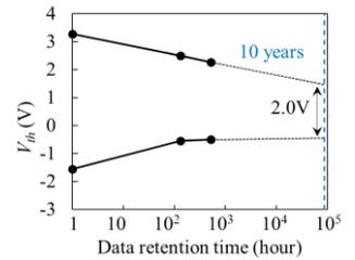
Fig. 13. Retention characteristics of FinFET SG-MONOS after 250K cycles at high temperature (150 °C).
