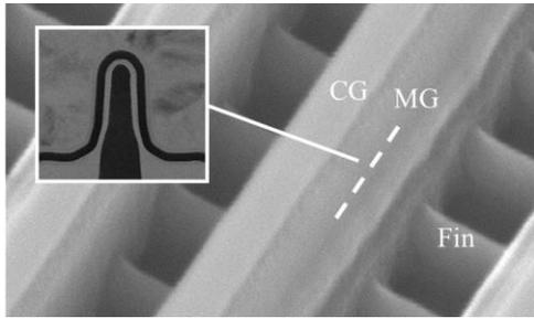
Fig. 3. Bird's-eye view of SEM image of FinFET SG-MONOS and Cross-sectional TEM image of MG-MOS.
