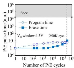
Fig. 12. Endurance characteristics of FinFET SG-MONOS.
