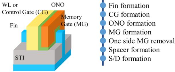
Fig. 1. Schematic view of FinFET SG-MONOS.
