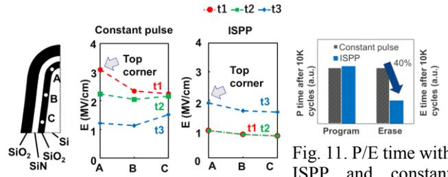
Fig. 10. Simulated electric field for constant pulse and ISPP.
