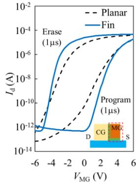
Fig. 5. I-V characteristics of MG-MOS at program and erase (P/E) states.
