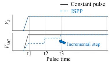
Fig. 9. Pulse diagram of constant pulse and incremental step pulse programming (ISPP).
