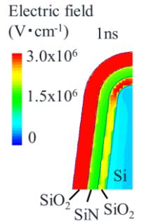
Fig. 8. Simulated electric field during program operation.
