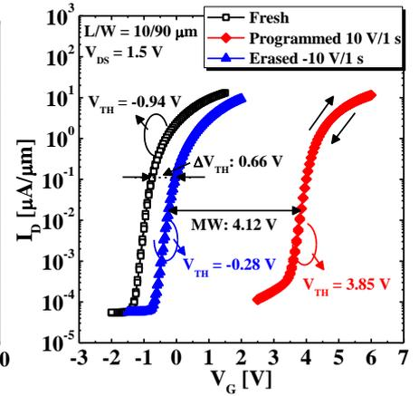
Fig. 5. I<sub>D</sub>-V<sub>G</sub> of in-situ formed Hf-based MONOS NVM.  $V_{PGM}/t_{PGM}$  was 10 V/1 s and  $V_{ERS}/t_{ERS}$  was -10 V/1 s.
