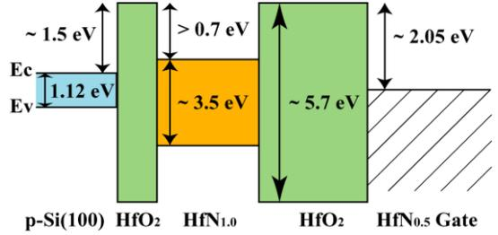
Fig. 3. Schematic energy band diagram of Hf-based MONOS structure.
