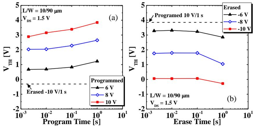
Fig. 7. Pulse width and voltage dependence on  $V_{TH}$ . Black dash lines denote  $V_{TH}$  before program or erase operation. (a) Program characteristics and (b) erase characteristics.
