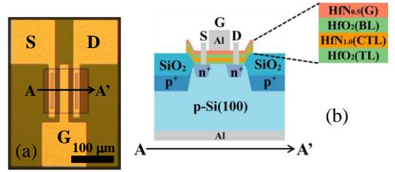
Fig. 2. (a) Plane-view and (b) Schematic cross-section (A-A') of in-situ formed Hf-based MONOS NVM.
