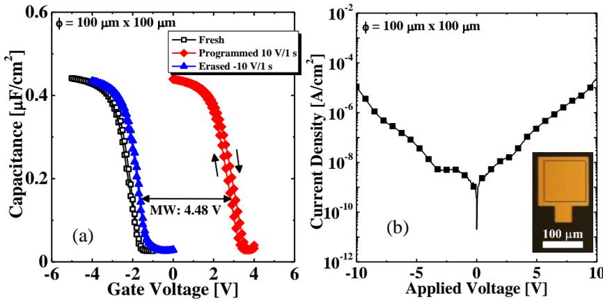
Fig. 4. (a) C-V characteristics of MONOS diodes.  $V_{PGM}/t_{PGM}$  was 10 V/1 s and  $V_{ERS}/t_{ERS}$  was -10 V/1 s. and (b) J-V characteristics. The inset in Fig. 4 (b) shows a top view of TEG
