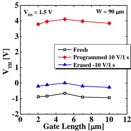
Fig. 6. Gate length dependence on  $V_{TH}$ . (L/W = 2-10/90 μm)
