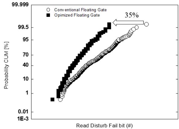
Fig. 6 Optimized floating gate has better read disturb characteristics.
