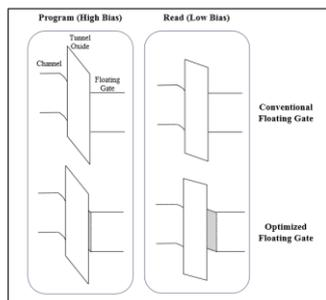
Fig. 4 Band diagram of conventional floating gate and optimized floating gate
