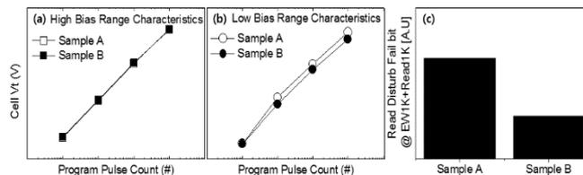
Fig. 1 Program characteristics under various program bias and pulse count, and read disturb characteristics of each sample.
