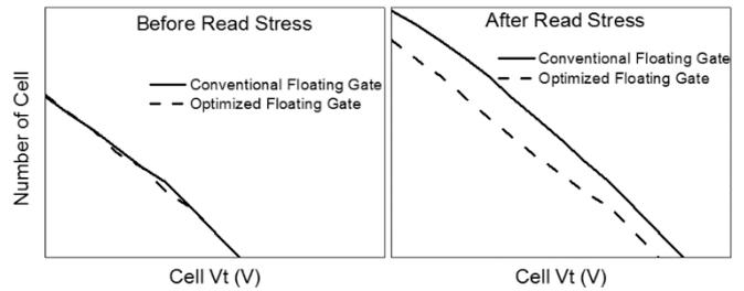
Fig. 5 Erased cell Vt distribution of conventional floating gate and optimized floating gate. Optimized floating gate has smaller shift than conventional floating gate after read stress.
