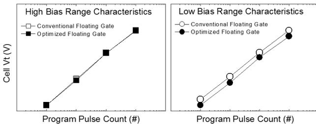
Fig. 3 Program characteristics of optimized floating gate
