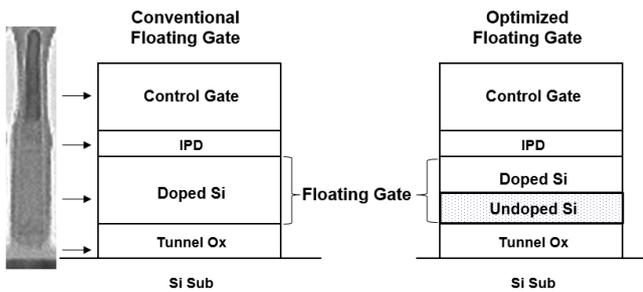
Fig. 2 Schematic structure of conventional floating gate and optimized floating gate.
