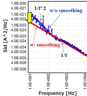
Fig. 6. Current noise intensity with and without smoothing along  $1/f$  slope.
