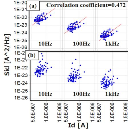
Fig. 7. The correlation of  $Id$  and  $Sid$  at  $V_g=V_{th}$ ; (a) with smoothed  $Sid$ , (b) without smoothed  $Sid$ .
