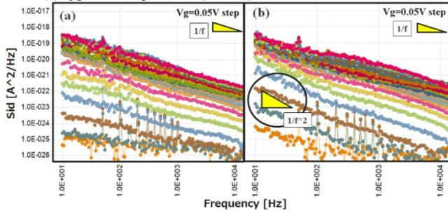
Fig. 5.  $1/f$  noise characteristics for various gate voltage condition. (a) typical sample data (bulk) (b) tail sample data (bulk) (c) typical sample data (SOTB)
