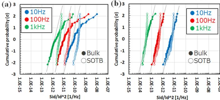
Fig. 3. Cumulative frequency distribution of normalized current noise intensity ( $Sid/Id$ ) in bulk and SOTB MOSFET; (a) weak inversion state, (b) strong inversion state.
