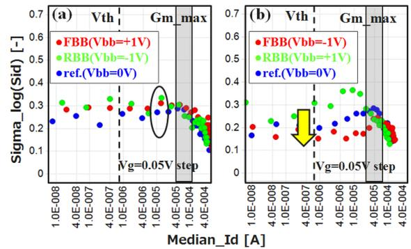
Fig. 10.  $Id$  dependence of  $Sid$  variability in SOTB MOSFETs at several back-gate voltages at 10Hz; (a) NMOSFETs and (b) PMOSFETs
