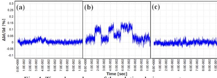
Fig. 4. Time dependence of the relative drain current (a) typical sample data (bulk), (b) tail sample data (bulk) (c) typical sample data (SOTB)
