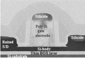
Fig. 1. Cross-sectional TEM image of SOTB MOSFET.
