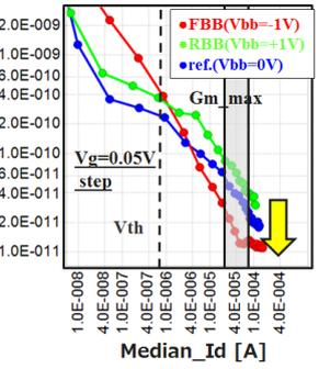
Fig. 11.  $Id$  dependence of  $Sid$  in SOTB PMOSFETs at several back-gate voltages at 10Hz.
