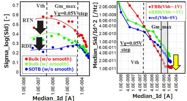
Fig. 9.  $Id$  dependence of  $Sid$  variability in NMOSFETs at 10Hz.
