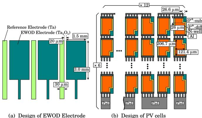
Fig. 2 The design of EWOD electrodes and PV cells. The EWOD electrodes are designed to carry a 50  $\mu$ L droplet. The PV cells are composed of 72 cells connected in series.
