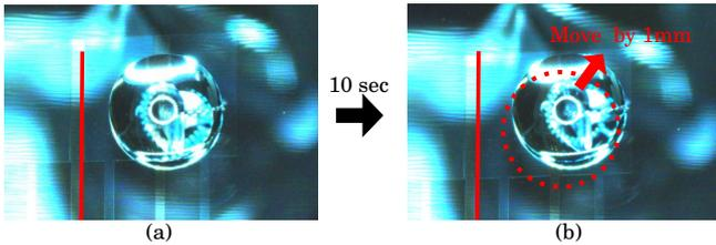
Fig. 5 (a) Initial position when the PV cells are illuminated (b) Position 10 sec after the PV cells are illuminated. One millimeter displacement was observed by illuminating the PV cell.
