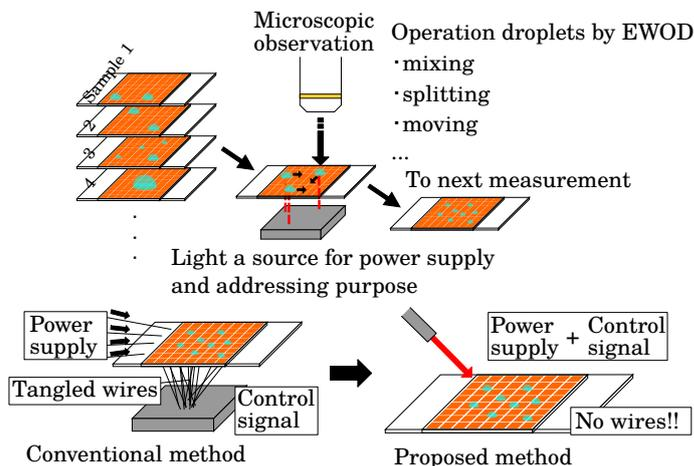
Fig. 1 A concept of wireless operation of EWOD microfluidics device
