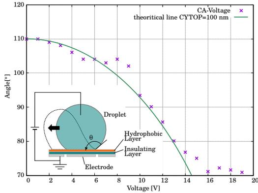
Fig. 4 The dependence of a contact angle at the liquid-solid interface on the applied voltage.
