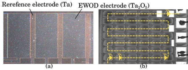
Fig. 3 (a) Microscopic image of the EWOD electrodes. (b) Microscopic image of the PV cells.
