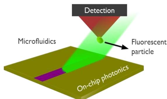
Fig. 1: Illustration of the miniature cytometry device indicating the photonics chip with specially designed grating (purple), created uniform illumination (green), fluorescent particle flowing through the microfluidic channel after being hydrodynamically focused, and its luminescence being detected (red).
