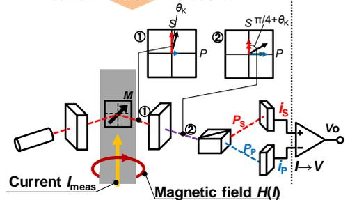
Fig. 2 Block diagram of the OPCS head [1,2].
