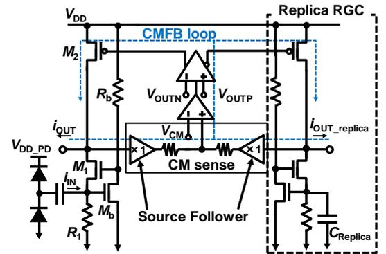
Fig. 4 Schematic of RGC amplifier stage.
