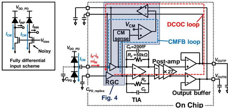
Fig. 3 Schematic of pseudo differential AFE circuit.
