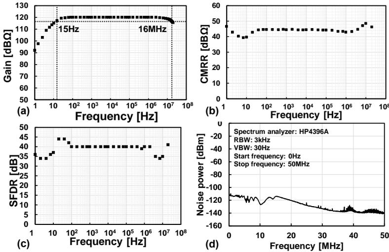
Fig. 6 Measured frequency response. (a) Gain (b) CMRR (c) SFDR (d) Noise power.
