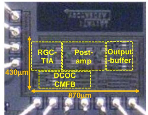
Fig. 5 Chip microphotograph.
