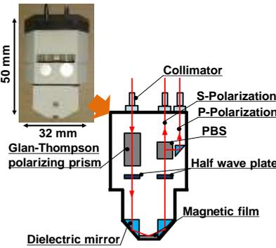
Fig. 1 Structure of the OPCS head [2].
